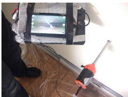
A borescope survey of a cavity wall showing the borescope inserted into the wall. The screen shows a tidy – and empty – cavity and a wall tie that is not straight.
